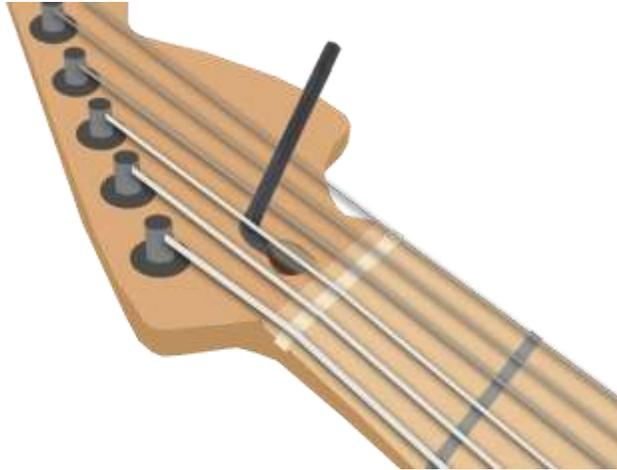
If there's a truss rod cover at the base of the headstock, remove the screws and take it off.
